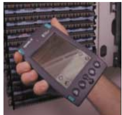
Supported by NDC's exclusive software, each component is scanned using Symbol Technologies' 1500 Bar Code Scanner-enabled Palm Pilot.
